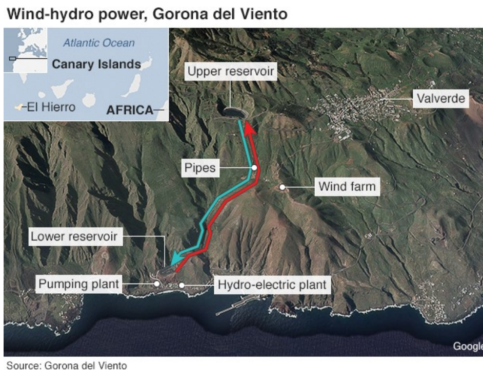
Fig.1 Layout of the Gorona del Viento electric production system. Not shown on the picture is the Llanos Blancos diesel plant located near the coast close to the pumping plant.
